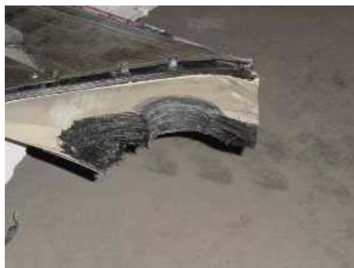
Below: One of the Vertical Stabilizer's Attachment Points
