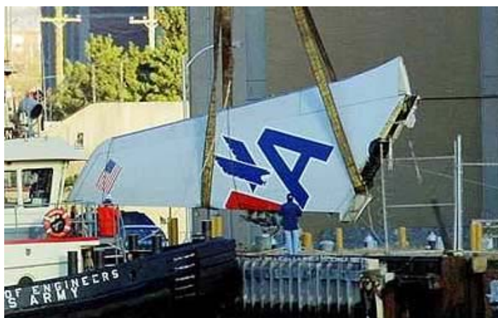
Above: Flight 587 Vertical Stabilizer Being Recovered
