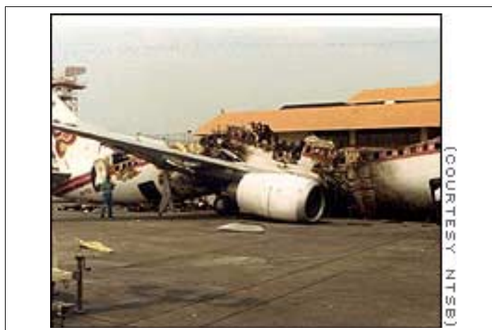
A spark caused by dry operation of the center tank fuel pump is the primary suspect in the deadly explosion.
